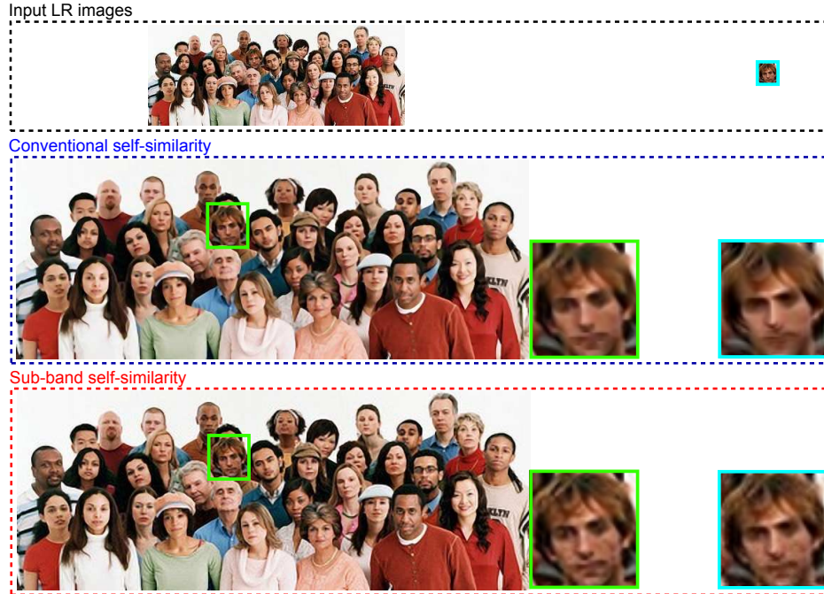
Fig. 13. An example showing the performance of our algorithm for very small input images. We super-resolve the two images shown in the black dotted box, the right one being a one face sub-image cropped from the left image. Our algorithm is able to super-resolve this small face image much better than the conventional self-similarity approach of [6].
