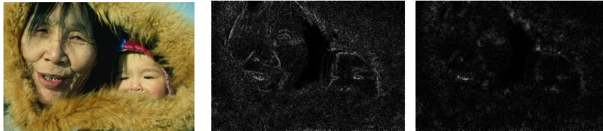
Fig. 3. Left: Input image. Center: Image indicating the errors obtained using conventional nearest neighbor search for each image patch, in the internal LR dictionary \mathcal{L} . Right: Corresponding error map obtained using the proposed sub-band based patch matching approach. Our approach yields lower matching errors, particularly around textural regions such as the fur around the faces.
